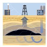
oll FROM SHALE Unlocking the shale is the latest energy imperative. Raytheon's idea is to free oil from rock by pumping liquid carbon dioxide into shale deposits heated up by lengthy blasts of radio waves.
