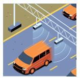
open-road tolling No searching for change, no waiting in lanes. Raytheon's toll road systems allow drivers with special transponders to pass under laser-equipped arches at or near the speed limit.
